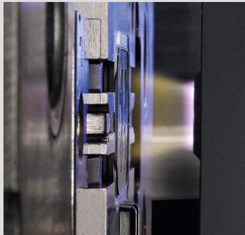
Fig. 1: The Openair plasma beam strikes the polycarbonate lenses with almost ultrasonic speed. Both the microfine cleaning effect and the high degree of activation impart the plastic material with new adhesion properties.
