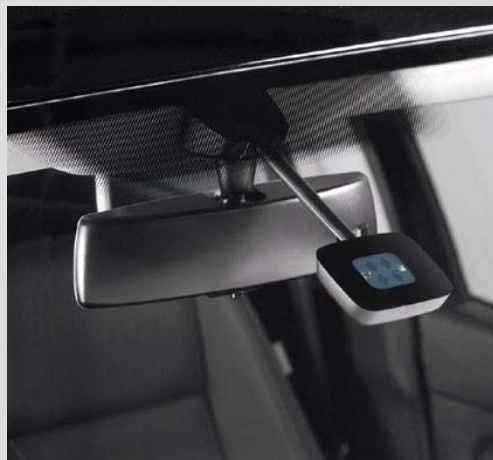
Fig. 2: The rain/light sensor reflects incoming light beams while measuring the light refraction. Transparent LSR forms the cover layer for adhesion to the glass pane.
