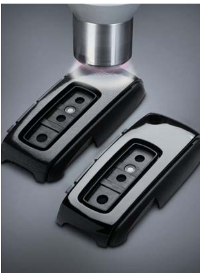
The part on the left shows the pretreatment of the PA key bottom shell with Openair plasma. The part on the right is the same part after application of the transparent scratch-resistant coating (Photos: Plasmamatreat)
