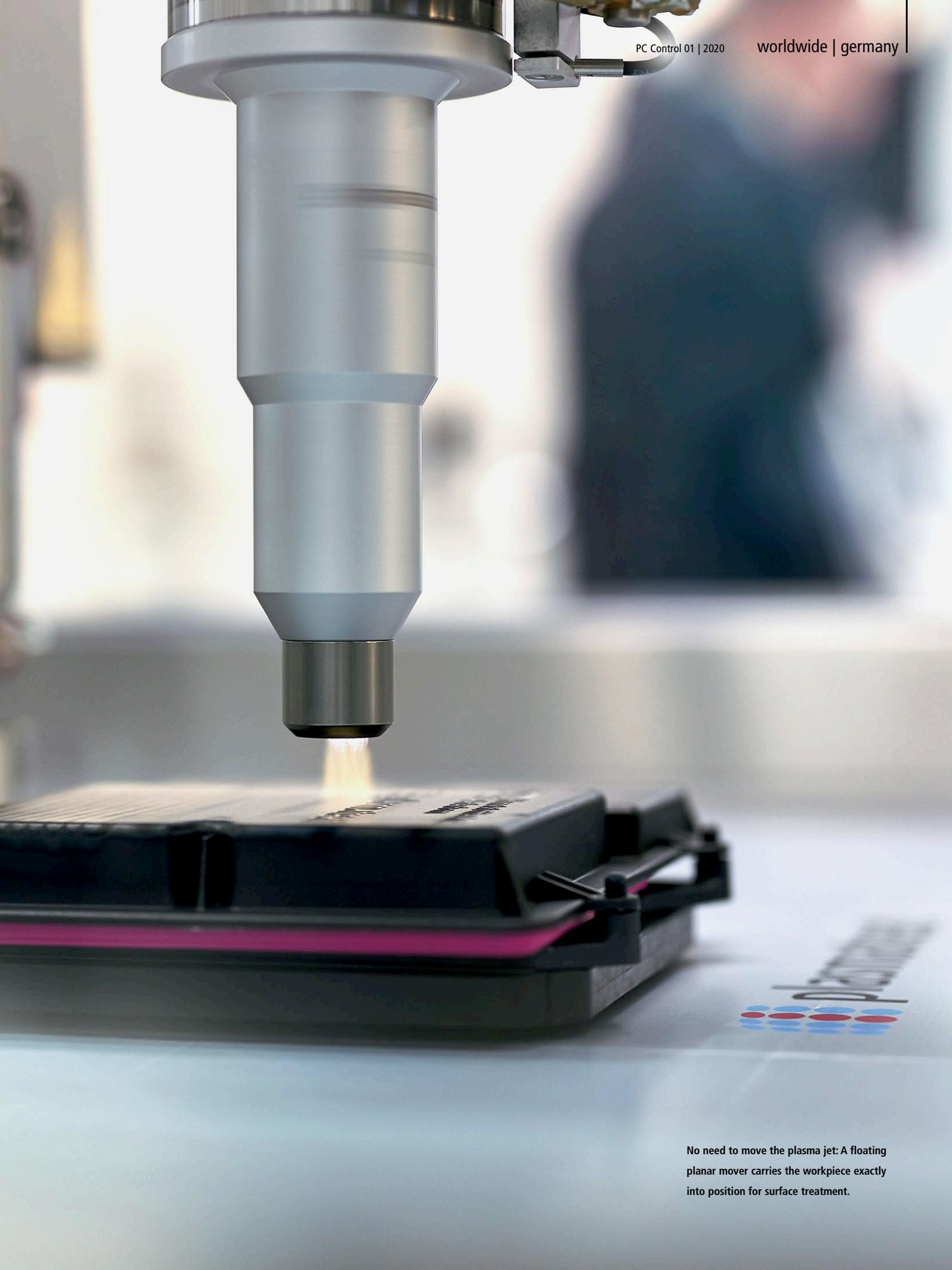
No need to move the plasma jet: A floating planar mover carries the workpiece exactly into position for surface treatment.
